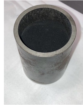
Figure 1. Green sand at ambient in 80 mm tall tube for permeability testing.
