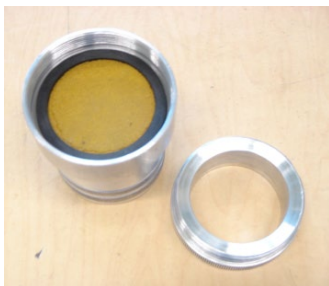
Figure 3. Disc-shaped specimen inside specimen holder.
